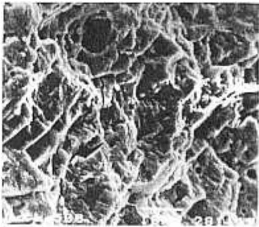
Fig. 15. SEM Fractography of as-sprayed sample.
