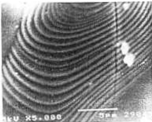
Fig. 9. Annealing twins on a higher post-heat treated sample (SEM).
