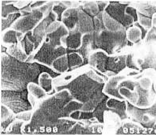
Fig. 18. SEM fractography of heat treated (1500 °C) sample.
