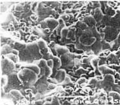
Fig. 8. SEM morphology of post-heat treated (1600 °C) sample.
