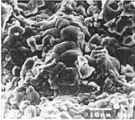
Fig. 17. SEM fractography of heat treated (1400 °C) sample
