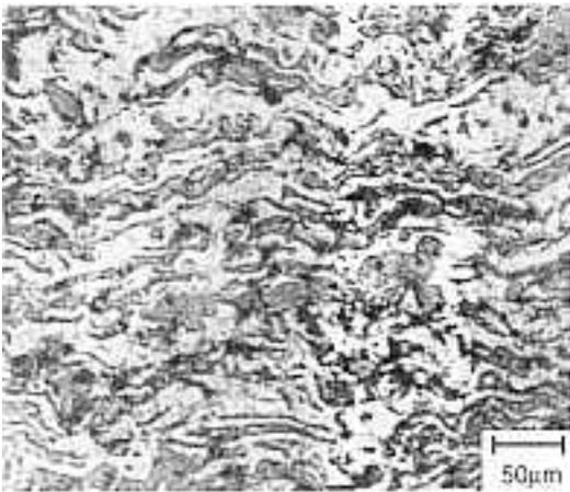
Fig. 2 Optical micrograph of cross-section of the as-sprayed sample.
