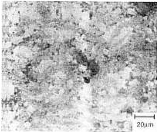
Fig. 5. Optical micrograph of the cross-section of a post-heat treated (1200 °C) sample.
