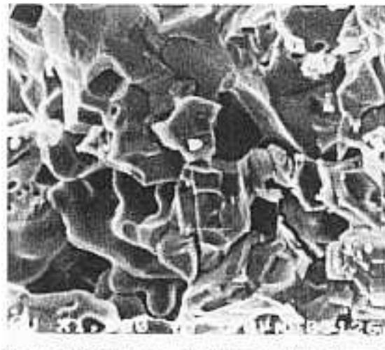
Fig. 19. SEM fractography of heat treated (1600 °C) sample
