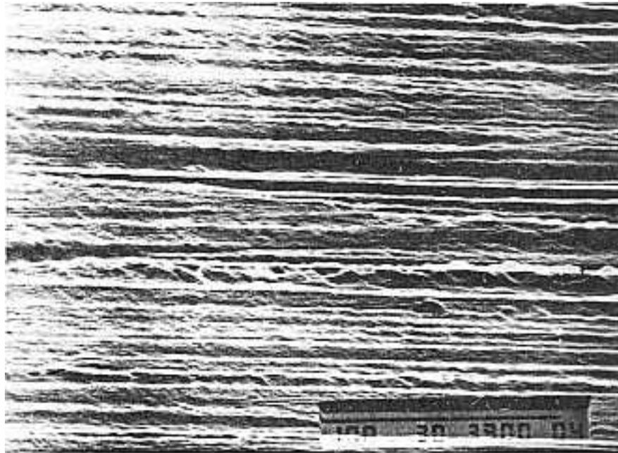
he scanning electron microscope (SEM) photograph of the ground-surface-as-sintered ceramic-ceramic composite in CBN wheel grinding at 3000 rpm and depth of cut 40  $\mu\text{m}$  at 500 x magnification.
